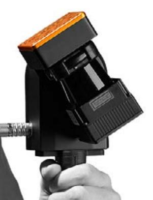
"Using the ZEB-REVO around 200 rooms were scanned, amounting to 12,000m<sup>2</sup>. Across 5 days, 12 individual rapid ZEB-REVO scans were completed each taking around half an hour. The entire project was completed in around half of the total time that would have been required using static equipment". Peter Maxwell, Midland Survey Ltd, UK
