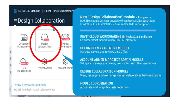
12.4 This is what you will see in Revit 2018.3 once you activate access to BIM 360 Design and initiate collaboration to the cloud. Revit 2018.3 is the Revit version in which you can collaborate in both, the new BIM 360 Design, as well as classic Collaboration for Revit with BIM 360 Team for data management.
