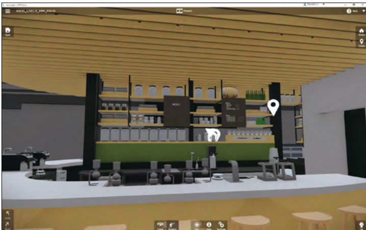
By using a head-mounted display, the 3D space can be experienced in VR and allows users to move around freely to check the design. [Provided by: Starbucks Coffee Japan]
