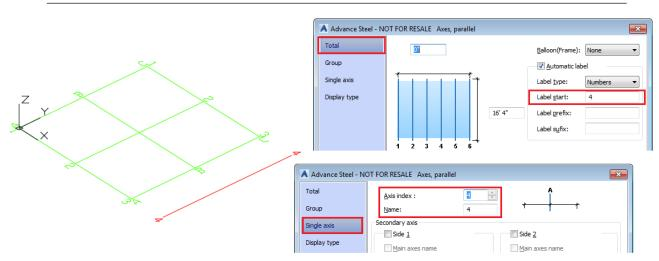
Next, extend the grid (the axis group created in the Y direction) to reach the newly created axis.
