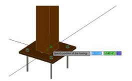
3. The isolated footing is created and the properties dialog box appears, where you can make the necessary settings.
