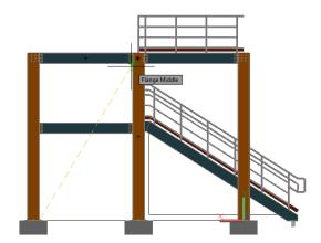
3. The bracing is placed and the properties dialog box appears, where you can make any required modifications to your bracing.
