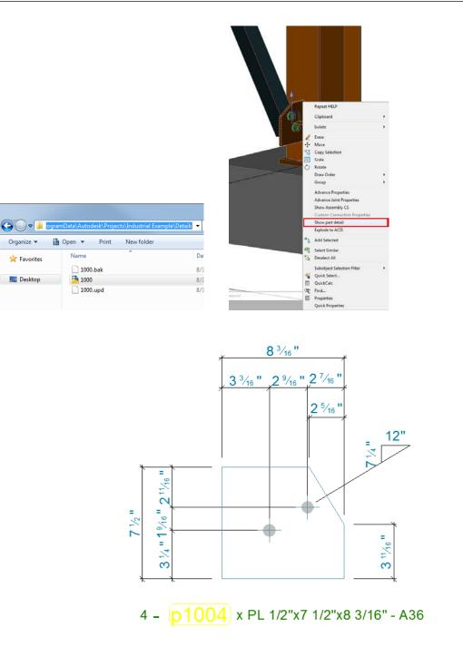
**Example:** Create a shop drawing with plates, using a drawing process.
